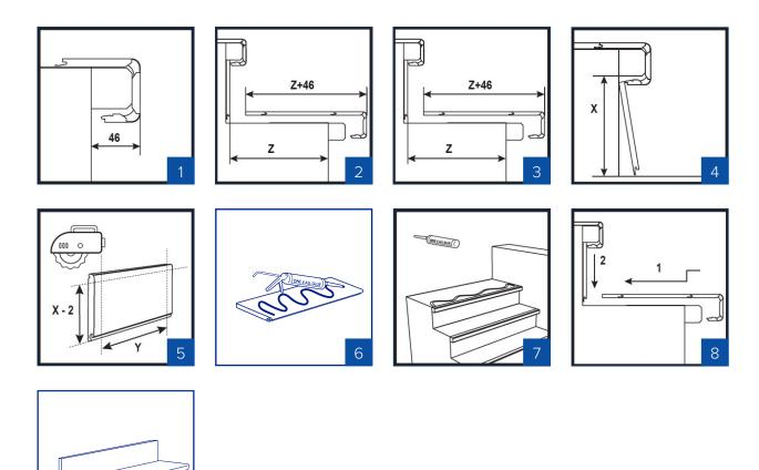
1. Measure the distance between the front of the Stair Cover and the below riser. < 46 mm: plank won't fit behind the Stair Cover. The bullnose must be enlarged or the Stair Cover adjusted to fit the floor plank for the riser and fully support the Stair Cover. ≥ 46 mm: check if you need to click an additional plank onto the bottomside of the Stair Cover to obtain a clean finish. Tape these two parts together on the backside and/or apply woodglue in the click profile.
