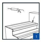
1. Finish seams with Quick-Step Coloured kit (QSKIT(-)) to hide any imperfections. The Coloured kit is available in white and different matching colours to your floor. The coloured kit is also paintable!
