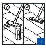
1. Maintain your finished staircase in the same way as your Quick-Step Laminate floor with our Quick-Step Floor cleaner. See quick-step.com for Laminate maintenance instructions.
